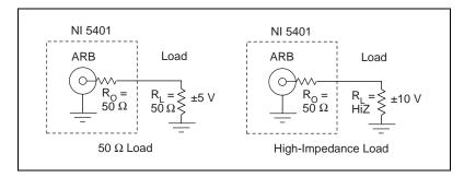
**Figure 1-2.** Output Levels and Load Termination Using a 50  $\Omega$  Output Impedance
